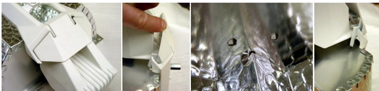
Using the lever to unlatch the reflector, aligning the notches with the reflector holes
