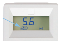
Successful pH 7 and pH 4 calibration
